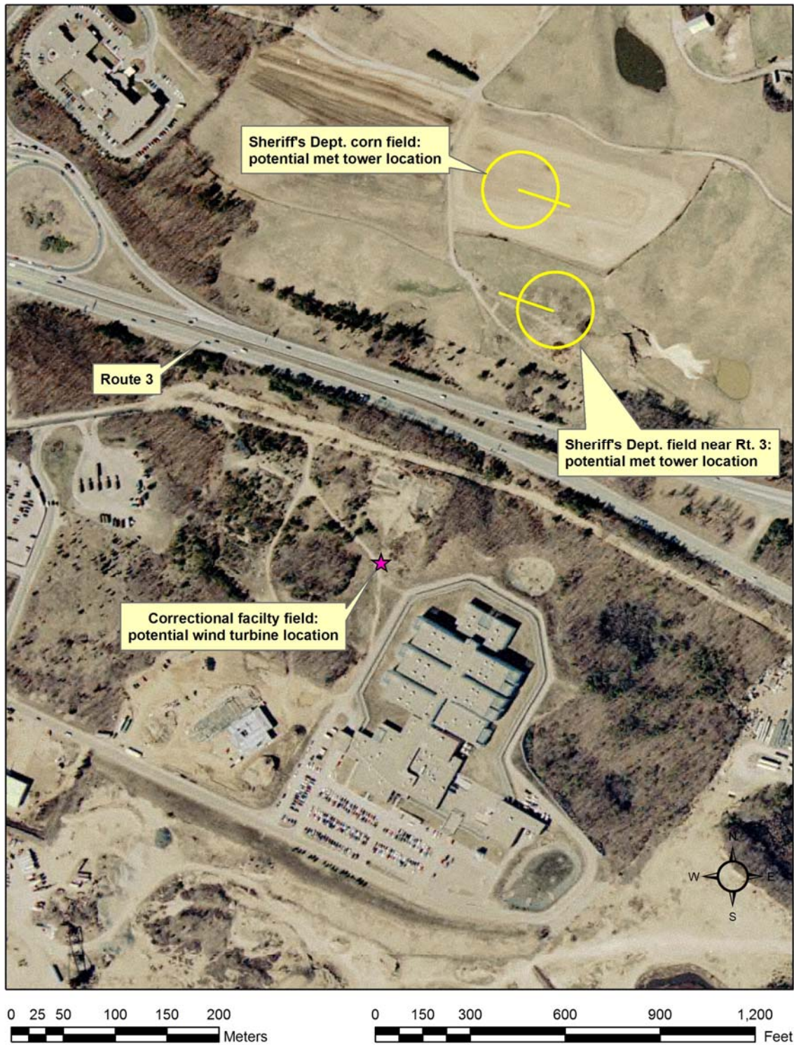
Map 3: This map shows 50-meter met tower layouts at the sheriff's farm fields.
